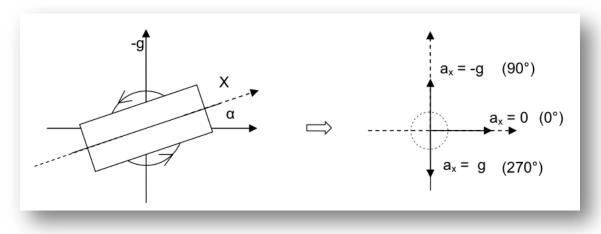
The X axis detects an acceleration equal to :
