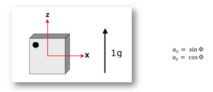
The use of two axes, one parallel and one perpendicular to  $\vec{g}$  allows to have a constant sensing  $\phi$  angle (on the plane x -z). This allows you to uniquely distinguish all the angle degrees.
