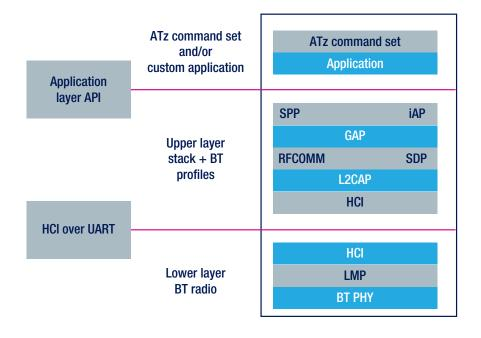
The new AT2 command set fully exploits the Bluetooth stack and efficiently supports communication with Android-smartphone and Apple iOS Bluetooth-enabled devices.
