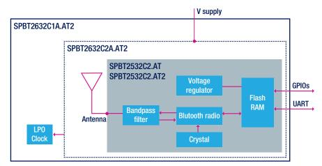
ST's new SPBT2632 offers a fullyintegrated and fully-qualified Bluetooth solution, ready to use with the smallest footprint available in a simple to handle SMD package.
