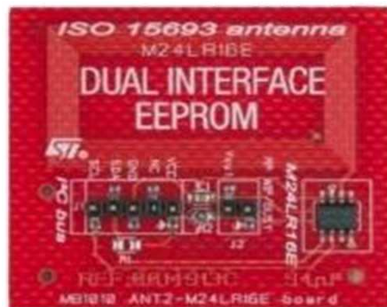
M24LR 40x20mm rectangular antenna
