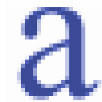
Generated character bitmap with color information (ARGB8888, ARGB1555, ARGB4444) or (RGB888, RGB565)
