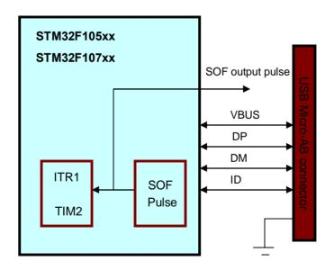
The USB SOF output for audio applications to synchronize the audio rate
